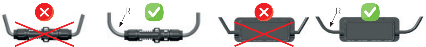
Fig. 5: permissible bending radius of the solar cables
